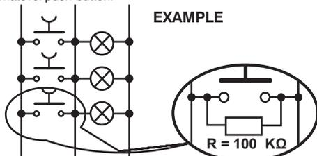
The working of the timed switch is subordinated to the connection to a minimum load (neon 40 W, electronic 16 W, incandescent 10 W) because, **in absence of load the product doesn't work**. When the connections are connected on the timer terminal board, the set time (from 30"  $\div$  7') will be automatically loaded. After the first cycle the insertion will take place by pressing the command buttons.
